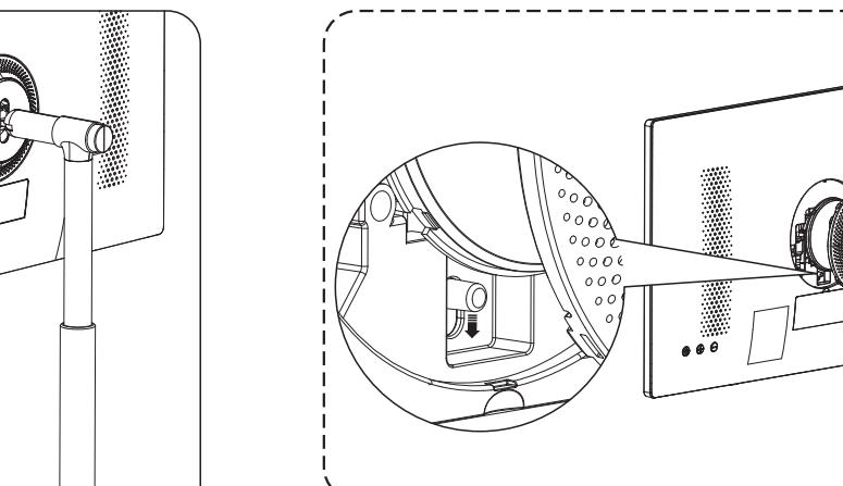
Attention: To disassemble, press the quick release button .
