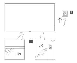
Plug one end (the two-hole plug) of the supplied detachable power cord into the power cord inlet on the rear side of the TV as shown above. Then plug the other end of the power cord into the mains socket outlet. The TV will switch to standby mode.
